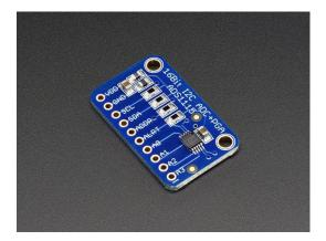
ADS1115 - 4 channel, 16 bit a/d with programmable gain amplifier
