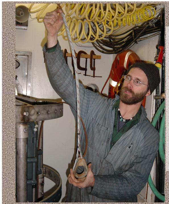
At this point, the grip termination (with or without thimble) has about 90% of the strength of the cable.
