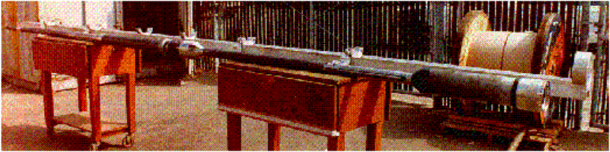
Plate 4b: The logging probe contains a camera, lights, navigation transponder, two calipers, and pressure and temperature transducers.
