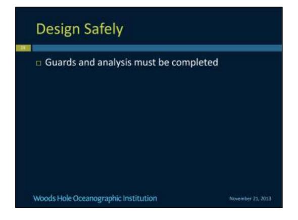
Around rotating machinery and finger pinches there should be guards as long as it doesn't impinge upon the operation of the equipment. An analysis should be completed for every piece of equipment.
