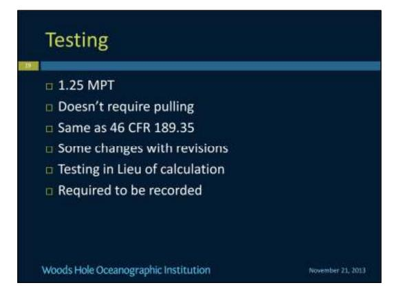
Testing is to 1.25 MPT. The equipment doesn't have to pull to 1.25 MPT. It can be achieved by chain fall or other apparatus. This is the same as the CFR. The new revision will have changes in the testing, including allowing testing instead of calculation. This is not the preferred method. It only provides the MPT not the DLT. All testing needs to be recorded and documented.
