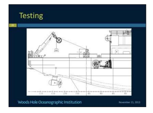
This test would only be for the winch and deck sockets. To test the a frame and block the frame should be out. This would then test the station keeping.
