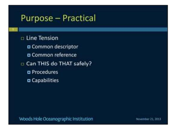
Provides a frame work using line tension as common denominator. Provides a common reference for equipment. This allows us to compare the capabilities of various components to tell if they are compatible, or what is the weakest link.
