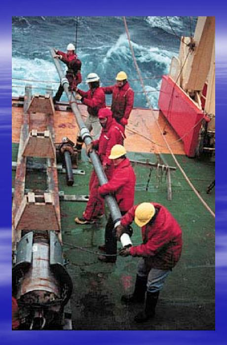
A piston corer that contains 24 feet of samples from the upper seafloor sediments
