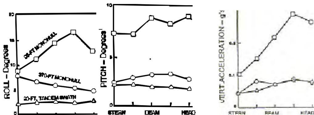
Fig. 2 - Comparative Performance of SWATH and Larger Monohulls
