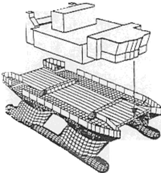
Fig. 6 - SWATH Carrier Vessel Concept
