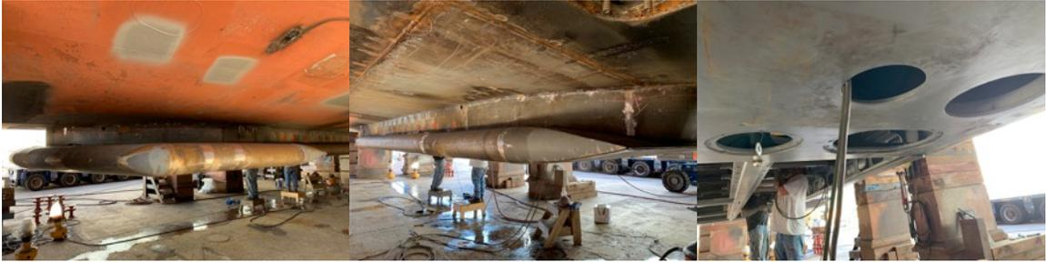
*Gondola installed and welded to hull and being prepared for painting*
