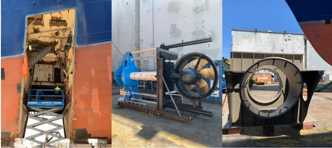
*Opening for thruster being prepped, new thruster, new thruster hull insert*
