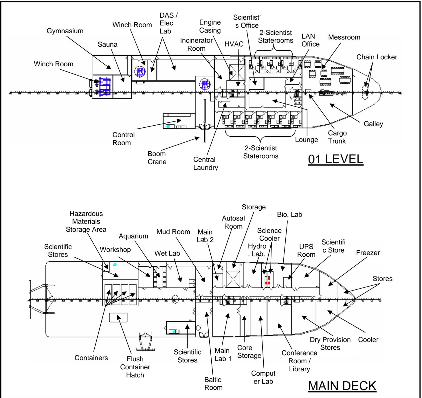
Fig. 6: PRV arrangements for the Main Deck and 01 Level
