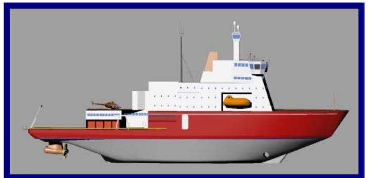
Fig. 8: Outboard profile of the PRV showing dual podded propulsors although traditional line shafting remains an alternative
