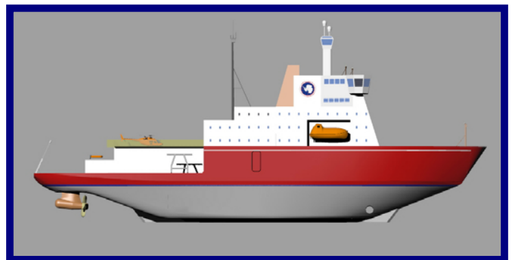
Figure 5. Outboard profile of the PRV showing dual podded propulsors
