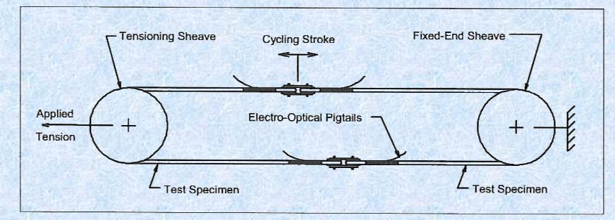
•Motor attached to one sheave to drive the samples.
