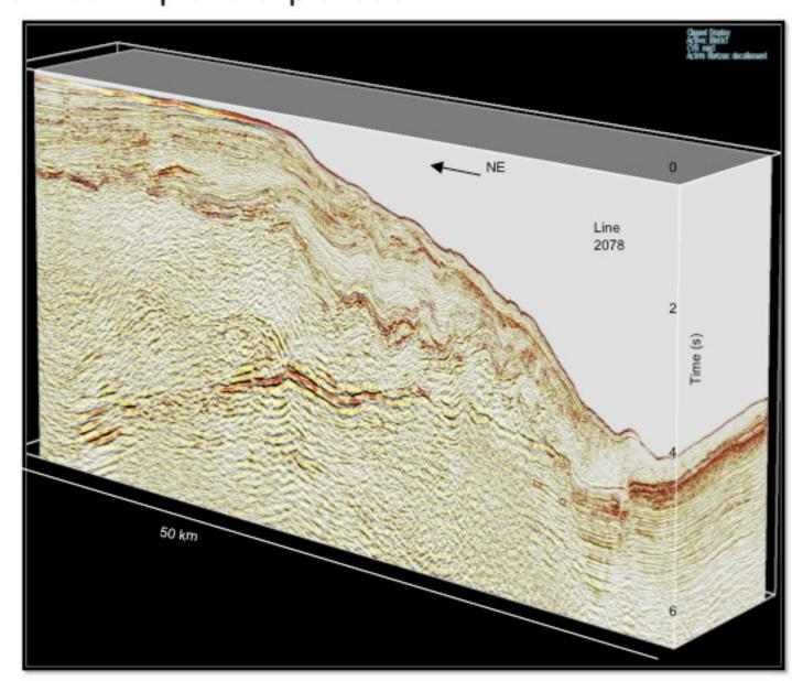
Regional 3D seismic profile through the Costa Rica margin from the shelf to trench. Low-amplitude values are in blue and high-amplitude values are from green to yellow.
