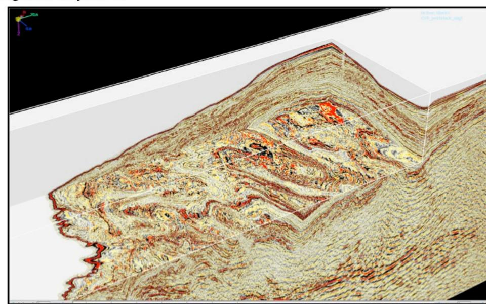
Subsurface '3D cube' of data with a horizontal time slice showing highamplitude anomalies.
