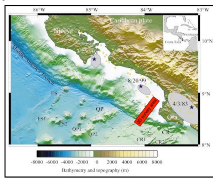
Topographic and bathymetric map of the Costa Rica subduction zone margin showing the location of the CRISP 3D seismic survey. The gray ovals are recent earthquake slip areas.
