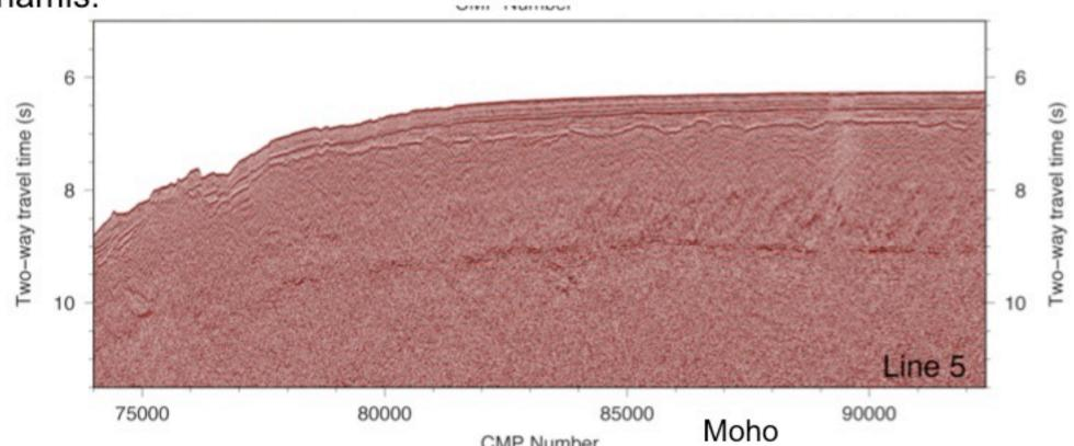
A close-up of the incoming oceanic plate, where we image extensive bending-related faulting as the plate subducts (left edge of the image). These faults are thought to be important for hydrating the oceanic lithosphere and bring water into the subduction zone. We also imaged interesting structures in the oceanic crust prior to subduction, including a bright Moho and dipping reflections in the lower crust (right portion of the image).
