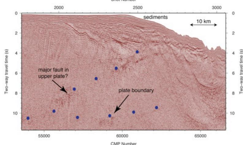
A close-up of a large fault that was imaged in the overriding plate, which is associated with a large basin and may connect to the megathrust. If this feature is active and connected to the plate boundary, it could be very important for understanding the potential for this region to produce tsunamis.
