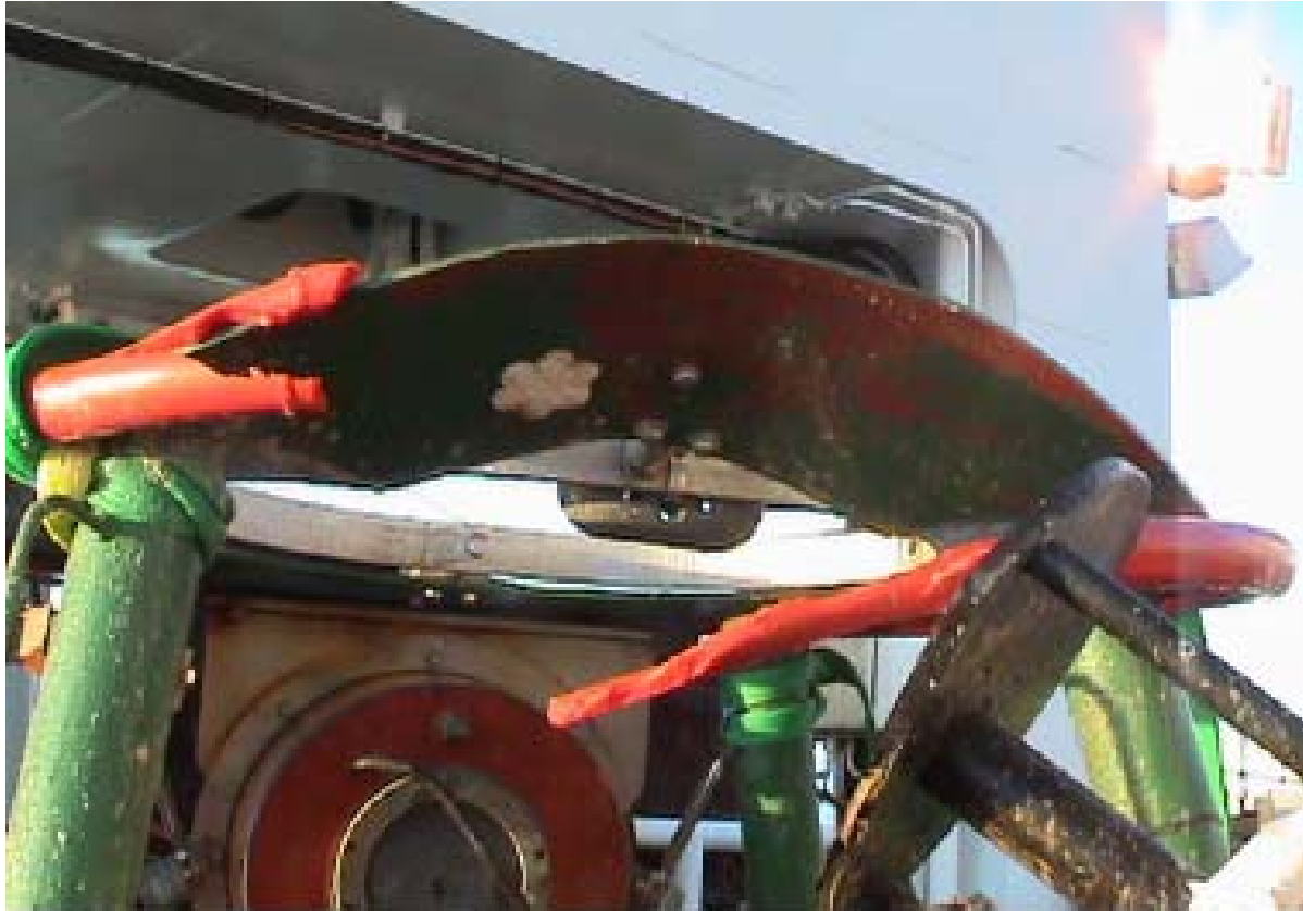
Top of lander: steel plates bended
