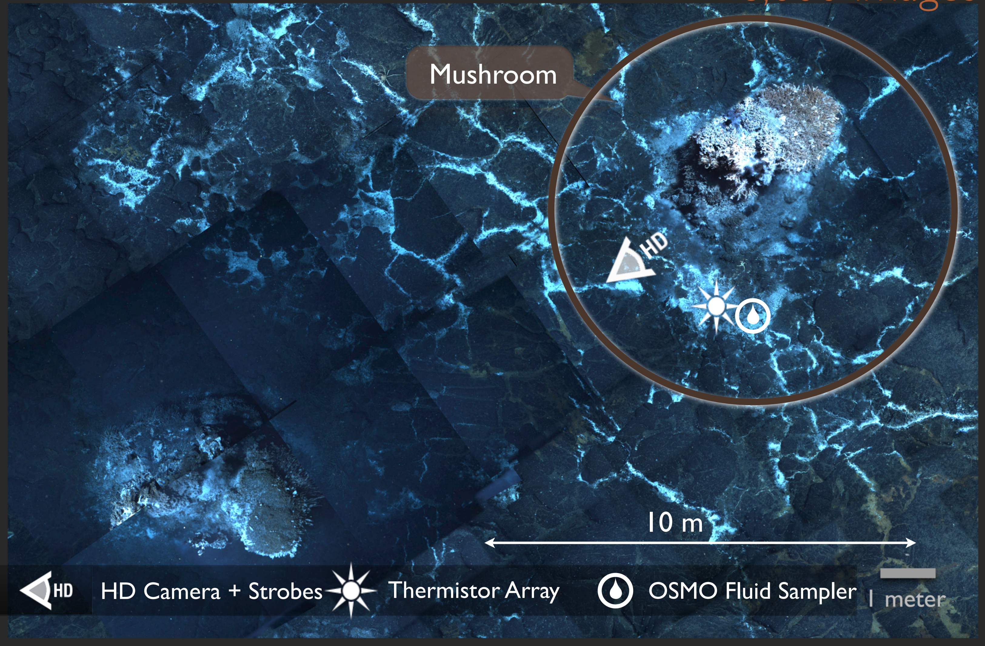
ASHES VENT FIELD: HD video, 3D temperature array, short-periods and fluid sampler will characterize changes in vent biology in response to changes in seismicity, temperature and chemistry
