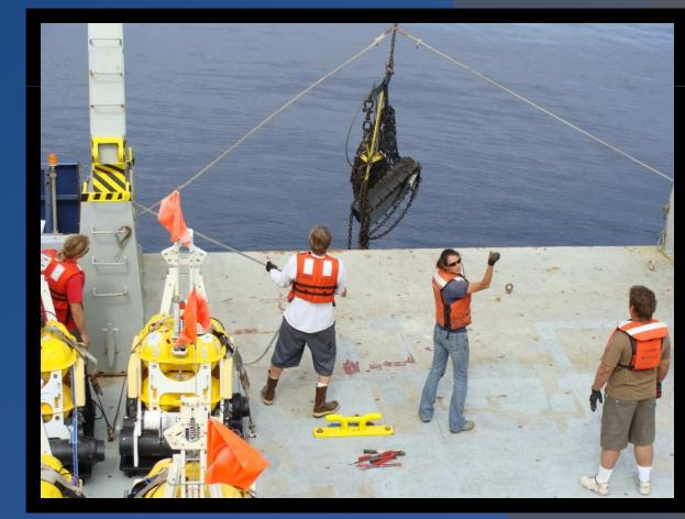
For dragging we employ variations on two techniques with two specific rigging set-ups. The "Check Mark" technique is typically used with Rigging #1. It is best suited for smaller items intended to be hooked or dislodged from the sea floor or release mechanisms. The "Lasso" technique coupled with Rigging #2 is best suited for mooring equipment recovery.
