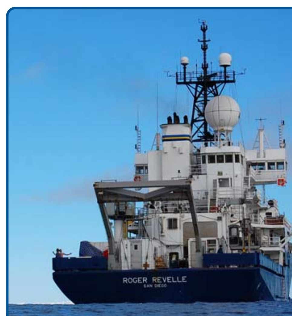
ABOVE: THE 274' R/V ROGER REVELLE EQUIPPED WITH A SEATEL 9797 2.4M ANTENNA (IN RADOME).
