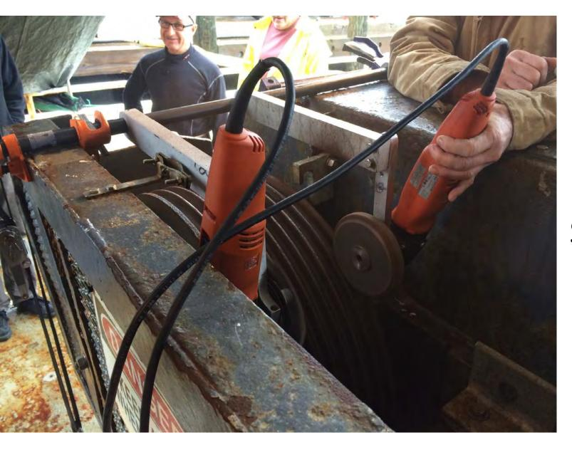
Pivoting grinders with wire wheels and Scotch-Brite discs
