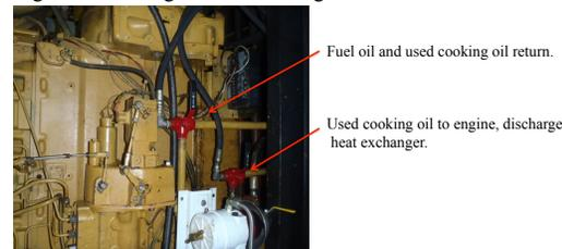
Figure 4. 3-way fuel oil / used cooking oil valves.
