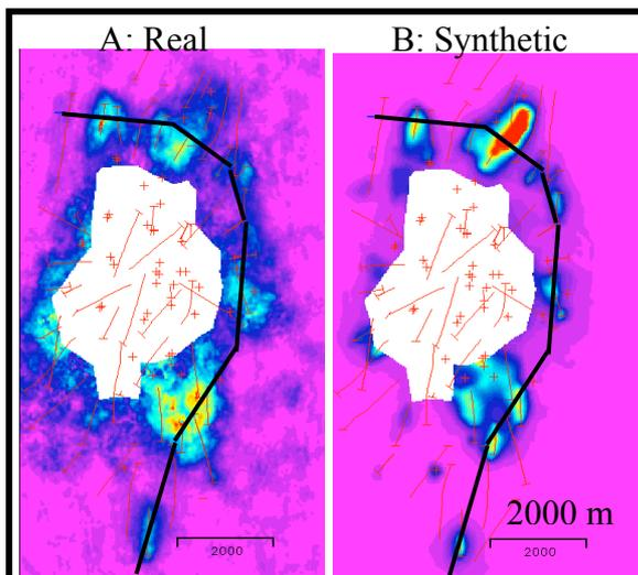
Figure 3: Top reservoir timeshifts calculated from the real (A) and synthetic seismic data (B). Timeshift color scale runs from 0 to 20 ms. The seismic traverse shown in Figs 1 and 2 is indicated by the irregular line.
