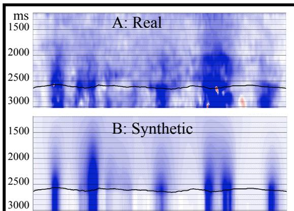
Figure 1: Cross-correlation timeshifts calculated from the real (A) and synthetic seismic data (B). Color scale to 10ms.
