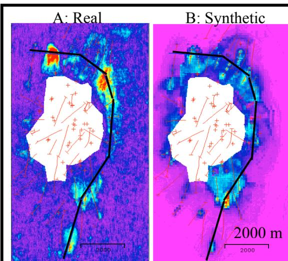
Figure 4: RMS amplitude measured at the top reservoir event from the real (A) and synthetic (B) shifted difference seismic.
