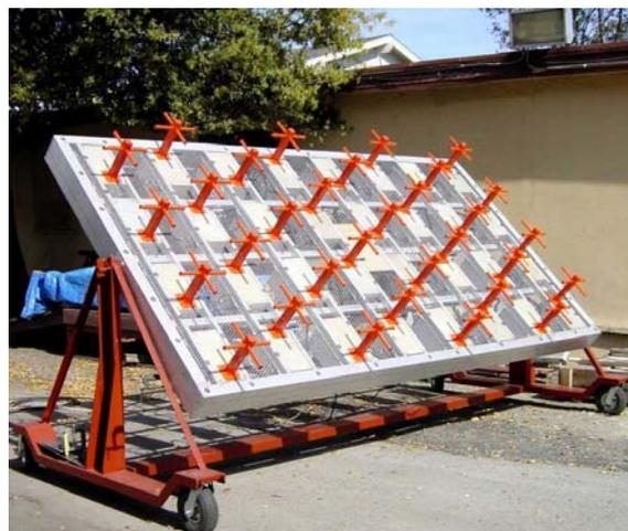
A single panel of 32 dipole antennas for the Advanced Modular Incoherent Scatter Radar (AMISR). AMISR consists of three antenna faces, each containing 128 of these panels. *Credit: SRI International*
