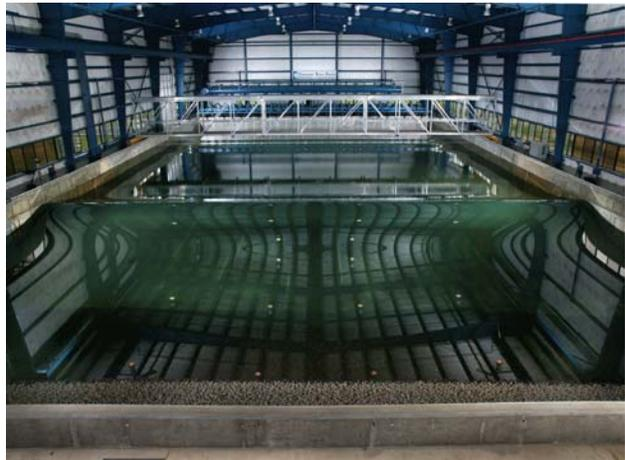
The NEES Tsunami Wave Basin is pictured above. Located at Oregon State University, it is the world's largest shared-use research facility for the study of effects of tsunami inundation on coastal buildings and lifeline infrastructures. A soliton (or solitary wave) is being demonstrated in this photo. *Credit: Kelly James, Oregon State*
