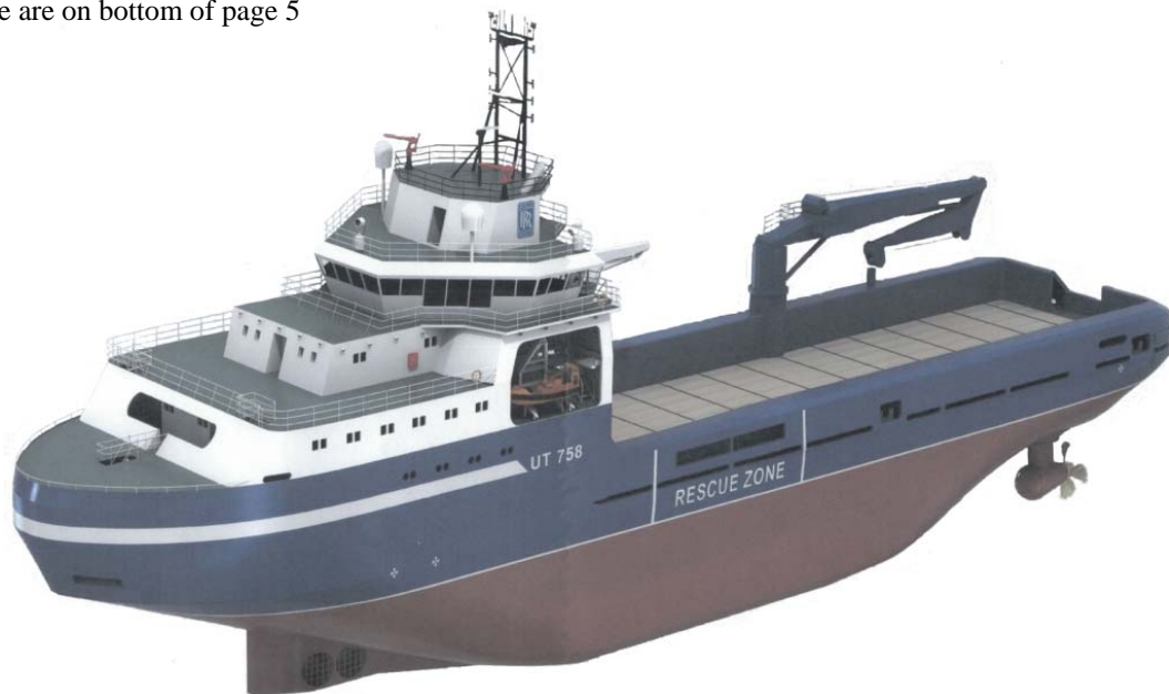
Three supply boats with 1.5 m (5 ft) icebreaking capability are being built in Norway. The UT 758 ICE was designed by Rolls Royce Marine AS
