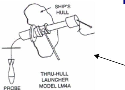
LM4A thru-hull launcher
