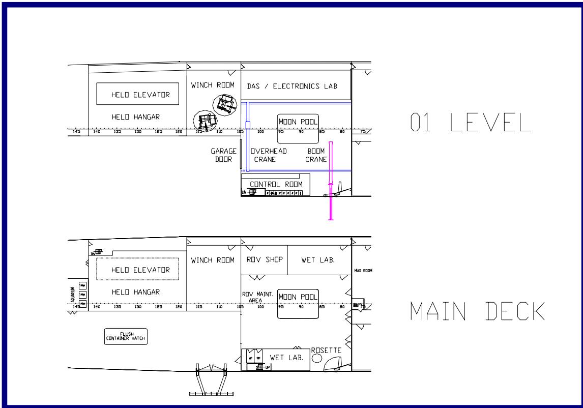
landing deck and a forward hangar had to be reconsidered. It appears that the most feasible solution was for the installation of an aft helicopter deck with a flush elevator for helicopter storage below. Sufficient space is provided such that two helicopters can be stored below on the Main Deck. This space is of sufficient size that it offers an excellent inside area for scientific vans when helicopters are not required aboard the vessel.
