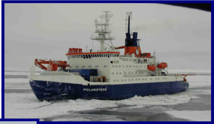
POLARSTERN (Length Overall 387 ft, Beam 82 ft, Draft 34 ft, Displacement 15,000 Tons and 17,000 Shaft Horsepower)
