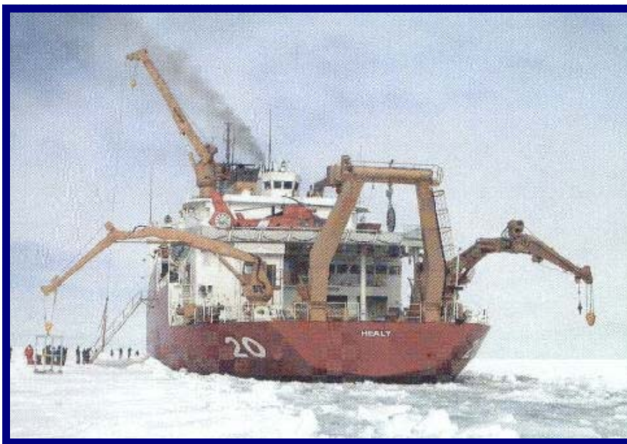
USCGC HEALY (Length Overall 420 ft, Beam 82 ft, Draft 29 ft 3 in, Displacement 16,000 Tons and 30,000 Shaft Horsepower)
