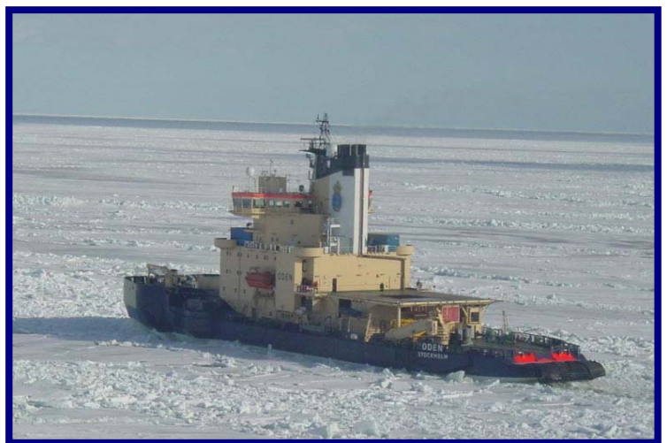
View of Swedish icebreaker ODEN (Length Overall 353.7 ft, Beam 101.7 ft, Draft 26 ft, Displacement 11,900 tons and 23,500 Shaft Horsepower)
