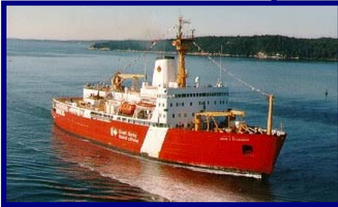
CCG LOUIS S. ST. LAURENT (Length Overall 892.5 ft, Beam 79.9 ft, Draft 32.5 ft, Displacement 14,500 Tons and 14,793 Shaft Horsepower)
