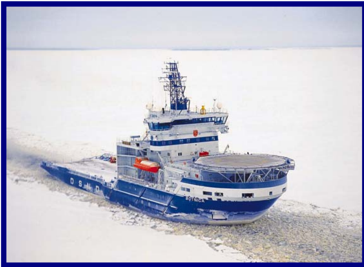
Finnish icebreaker BOTNICA in a broken ice channel (Length Overall 317 ft, Beam 78.7 ft, Draft 25.6 ft, Displacement 7,300 tons, and 13,500 Shaft Horsepower)
