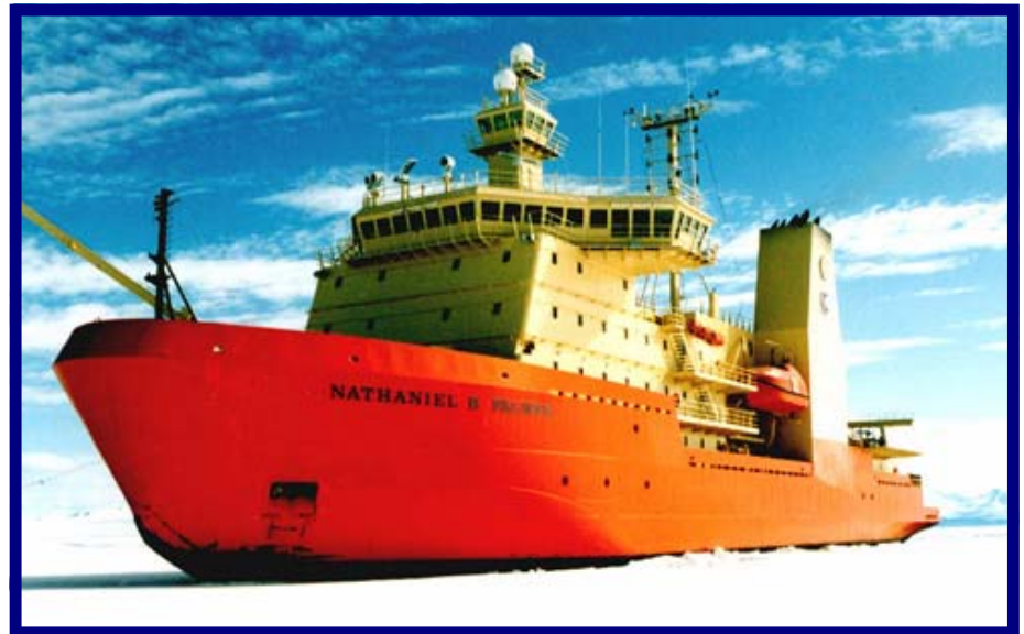
NATHANIEL B. PALMER (Length Overall 308 ft, Beam 60 ft, Draft 21.8 ft, Displacement 6,500 Tons and 13,200 Shaft Horsepower)
