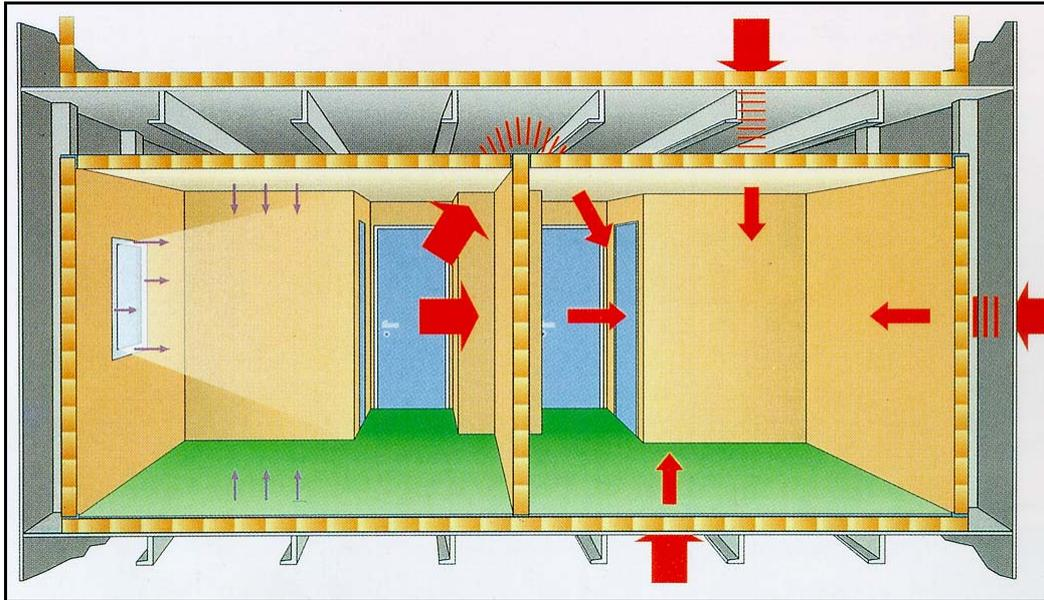
Figure D4: Generalised Schematic showing possible transmission paths into a cabin
