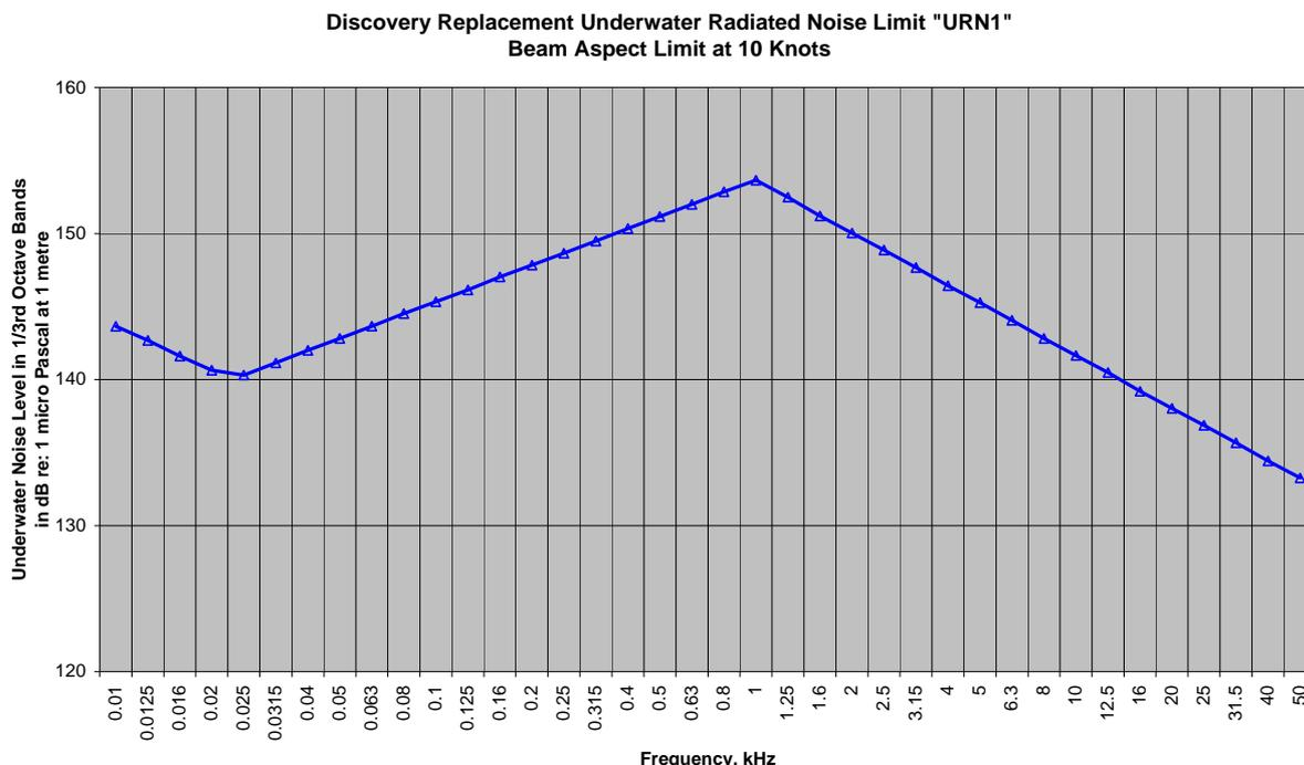
**FIGURE D1:** Underwater Noise Limit “URN1” for Beam Aspect of a **DC Motor** Driven Vessel when Free Running at all Vessel Speeds up to and including 10 Knots
