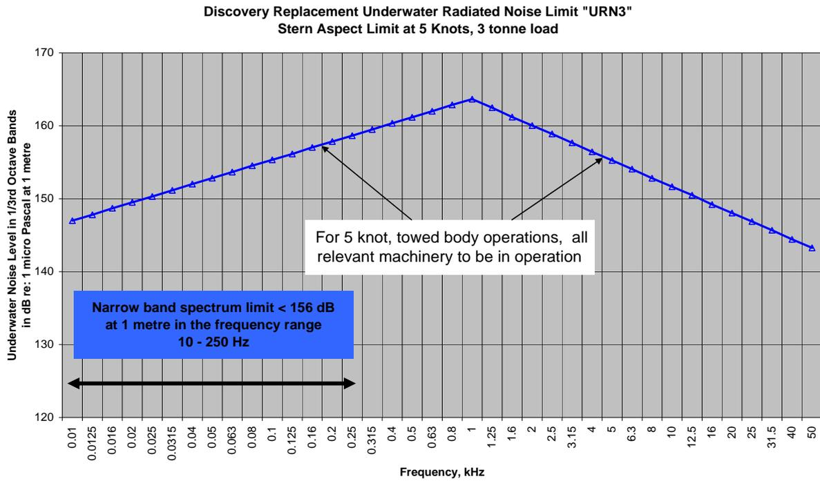
**FIGURE D3:** Underwater Noise Limit “URN3” for Stern Aspect of the Vessel when any Drive System (DC/AC/Azimuth) is used on the Vessel, whilst Towing a Load of 3 Tonnes at Vessel Speeds of up to 5 Knots
