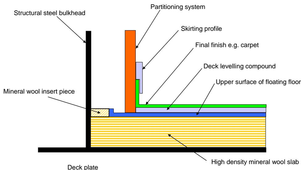
Figure D6: Generalised Schematic of Floating Floor showing Typical Edge Details
