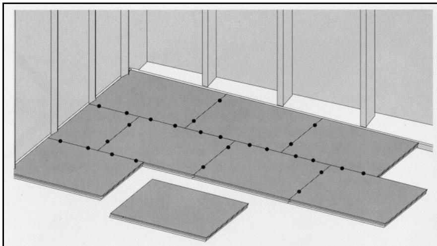
Figure D5: Generalised Schematic showing Floating Floor Slabs or Planks
