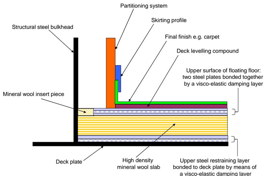
Figure D7: Generalised Schematic showing Constrained Layer Damping System on Deck combined with a high performance (damped) Floating Floor System
