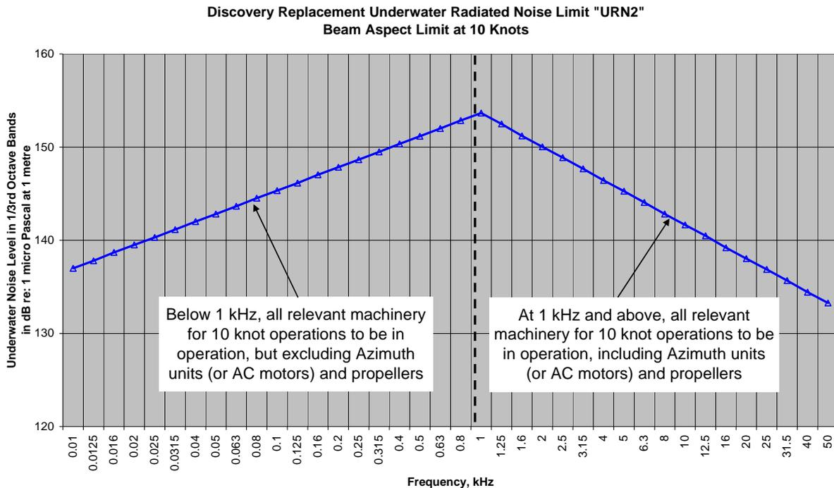
**FIGURE D2: Underwater Noise Limit “URN2” for Beam Aspect of Azimuth or AC Motor Driven Vessels** when Free Running at all Vessel Speeds up to and including 10 Knots
