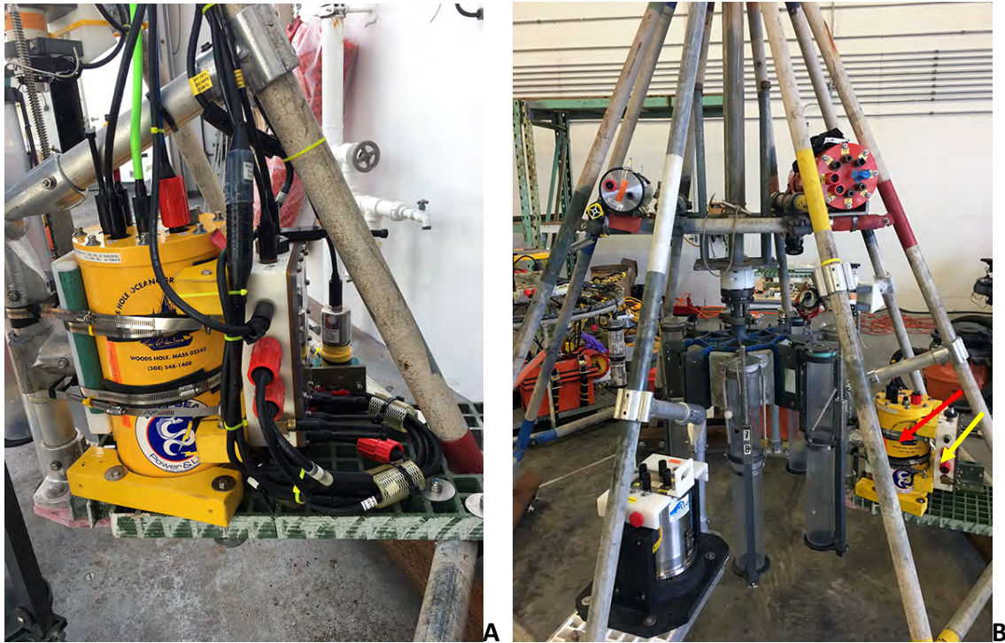
Figure 2. (A) MISO HD video recording system (large yellow housing, red arrow in B image) mounted on MC-800 platform, with power Junction Box (white box in middle of photo, yellow arrow in B image), and Valeport 500P altimeter/depth sensor (small, silver cylinder just to right of J-box). (B) Overall view of MC-800 with MISO equipment mounted – large orange housing on upper-right part of frame is the DataLink telemetry, smaller silver housing on left side is the strobe electronics (see Fig. 3).
