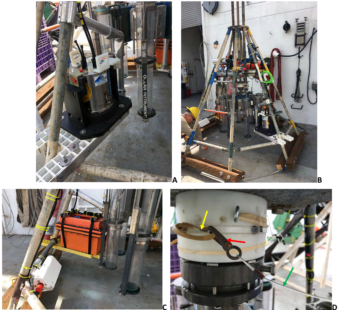
Figure 1. (A) 24MP OIS digital still camera mounted on platform on MC-800, top of image points towards center of core assembly. (B) Overall view of MC-800 with MISO imaging and data systems mounted. (C) Deep-sea battery mounted on platform (orange case) and one of the two strobe reflectors at lower left. (D) Anti-pretrip collar rigged. Brass clip (red arrow) attaches to the pull-loop (yellow arrow), the clip is attached to the monofilament line (green arrow) which runs to the winch motor that is triggered via the DataLink telemetry to remove the collar prior to landing the corer on the seafloor.
