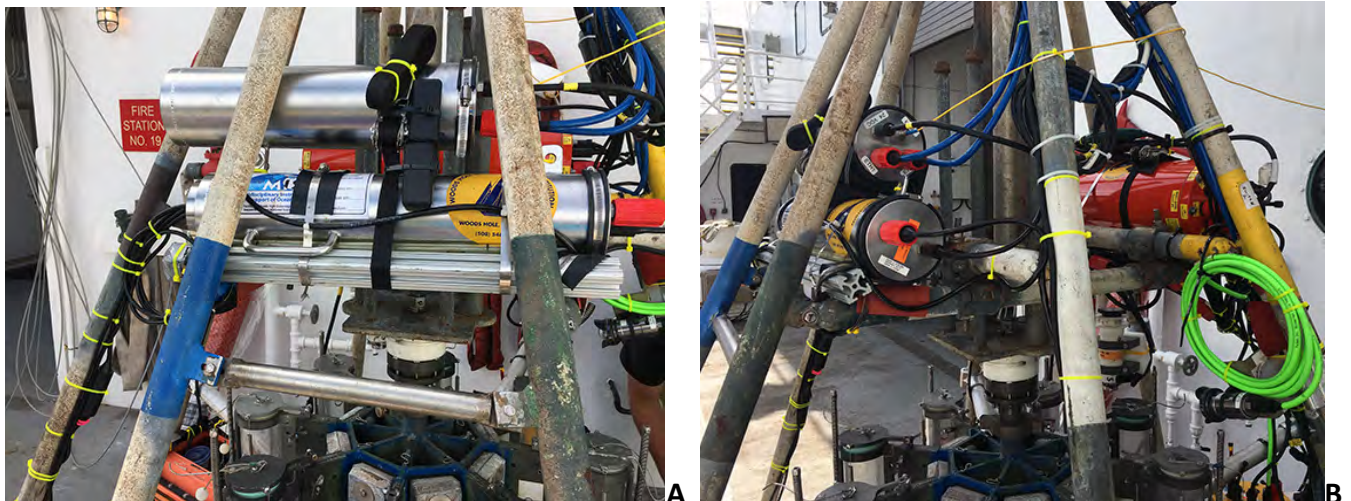
Figure 3. (A) Lower silver housing in middle of image is the 300 watt/sec strobe electronics, upper silver housing is the fiber optic to Ethernet converter electronics where the fiber connection from the cable is made with the two Ethernet ports providing connectivity to both the video system and the DataLink telemetry so that one can control the video on/off and LED light, as well as view the 24MP digital still camera r/t image and the depth/altitude 1 Hz data stream. (B) Side view on connector end of the strobe and fiber-to-Ethernet housings. Green cable at right edge is HD camera cable, just below the cable is the Deep-Sea Power & Light FlexLink HD camera.
