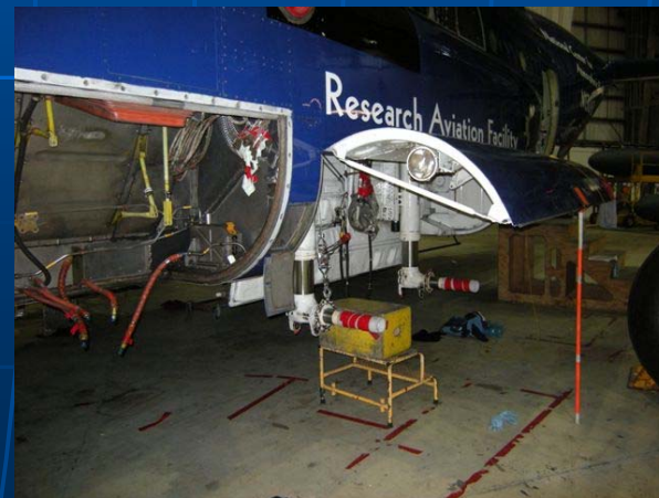
Major inspection of C-130
