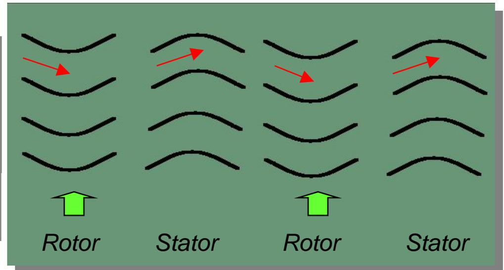
*The compressor compresses the air by accelerating and then decelerating it, since the pressure and the air speed are inversely proportional.*
