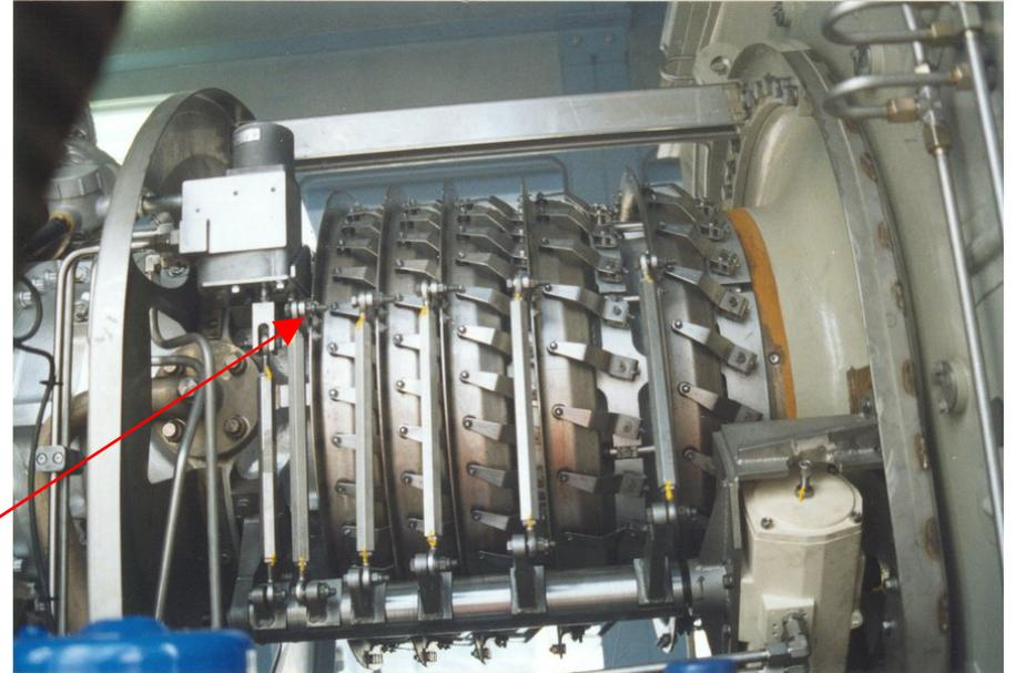
The Compressor compresses air by acceleration and deceleration, being pressure and air speed with inverted law.
