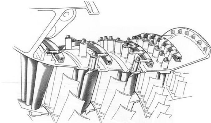
Compressor view: adjustable stator blades (IGV)
