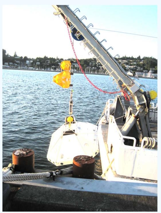
**Shield:** Eight-sided; 1/4" steel plate. Heavy (~700 kg in air) and with low, smooth profile to deflect trawling gear. No anchor left on seafloor.
