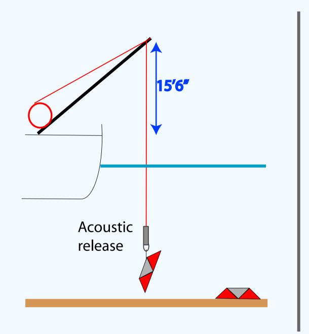
The heavy weight and low profile of the instrument preclude the use of dropweights for deployment and recovery. The OBS is instead lowered to the seafloor using a wire and acoustic release. It is recovered by attaching a lifting line using a remotely-operated vehicle (ROV). Instruments in water depths shallower than 170 m are equipped with popup buoy release systems.
