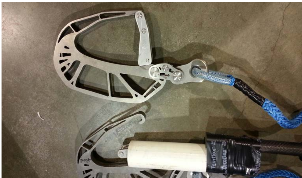
Titanium buoy pick up hook:
