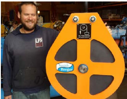
Hanging Block/Sheave – 34,000 DLT (with Chris Holm – on the left)
