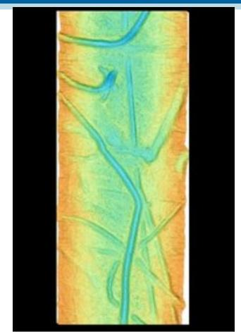
Processed multibeam data, showing iceberg gouges on the Chukchi Shelf. The depths are color-coded: Blue is deep and red is shallow. (Coakley, NY Times – Scientist@Work blog)
