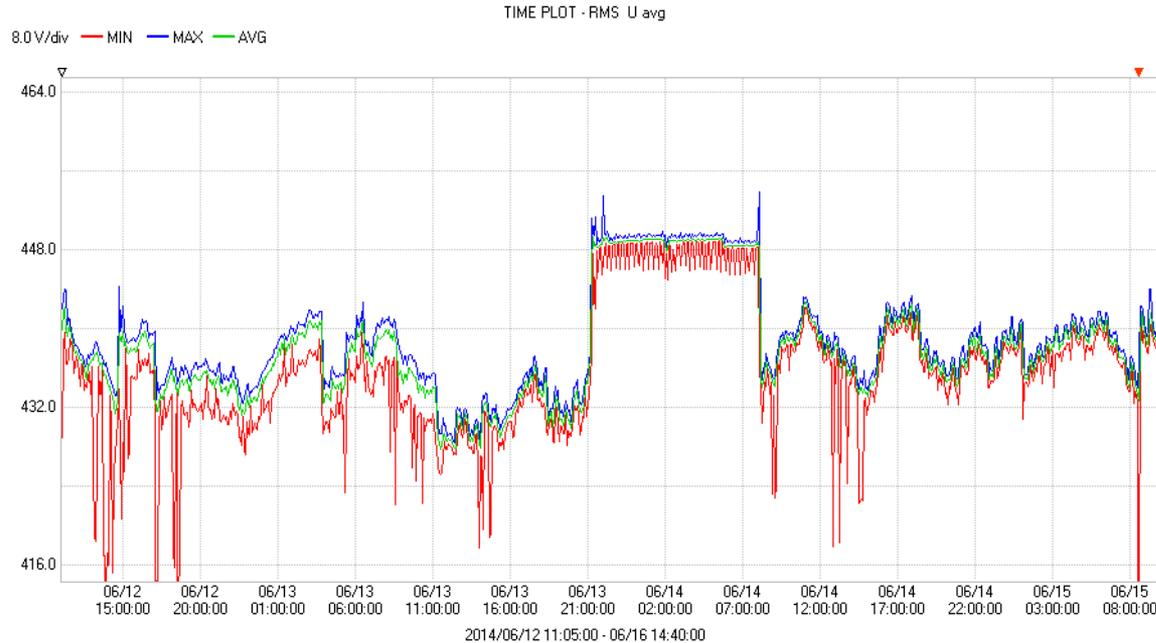
460 VAC Motor operating on low voltage (down to 426 VAC or 7% below name plate value) which increases motor slip causing decreased chiller capacity
