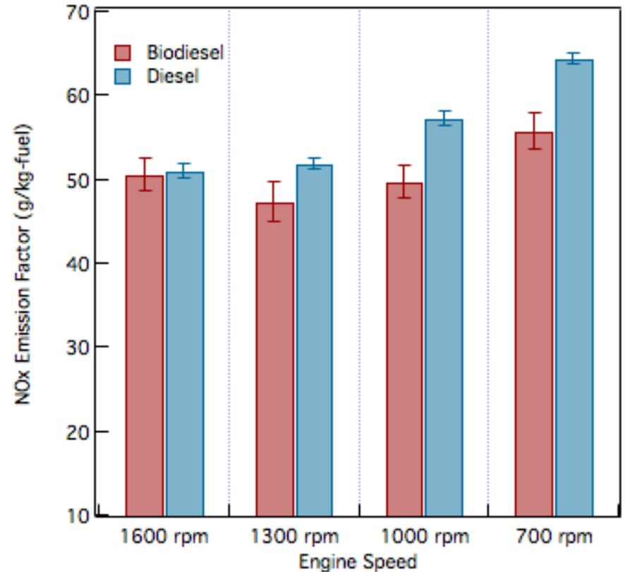
Emission factors of CO and NO<sub>x</sub> from R/V *Robert Gordon Sproul* at different engine speeds when powered by diesel and biodiesel. Each mean represents the average of a number of one-hour test periods (n=7 for biodiesel; n=2 for diesel). The average was calculated over different engine cycle tests conducted during a 2015 cruise.
