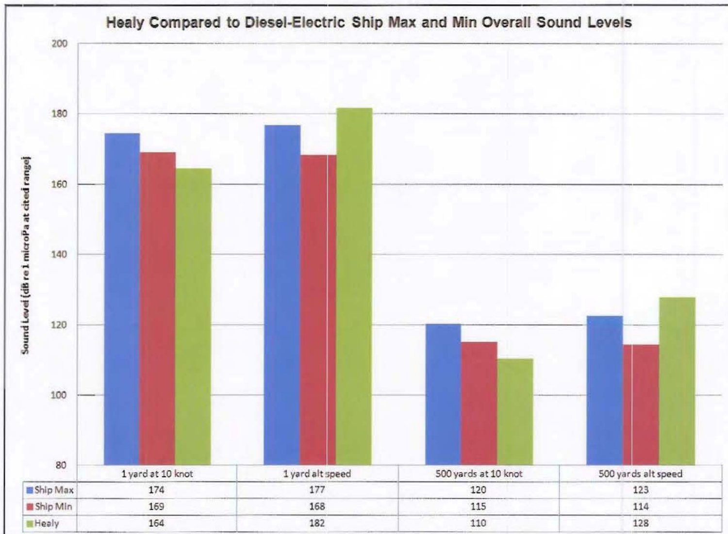
Figure 7. Healy Compared to Diesel-Electric Ship's Max and Min Overall Sound Levels at Range and Speed
