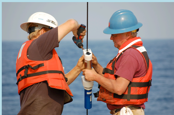
Figure 5. One of the 150 Hydrophone Modules that made up the 5000-m long DVLA receiver for the 2010–2011 NPAL Philippine Sea Experiment being recovered on the R/V Revelle . (Photo: L. Green, SIO.)
