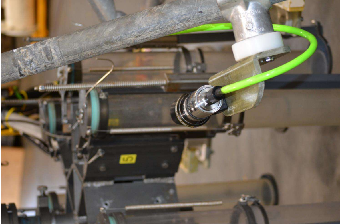
(right) 5L Niskin mounted on one of the vertical legs of the MC800
