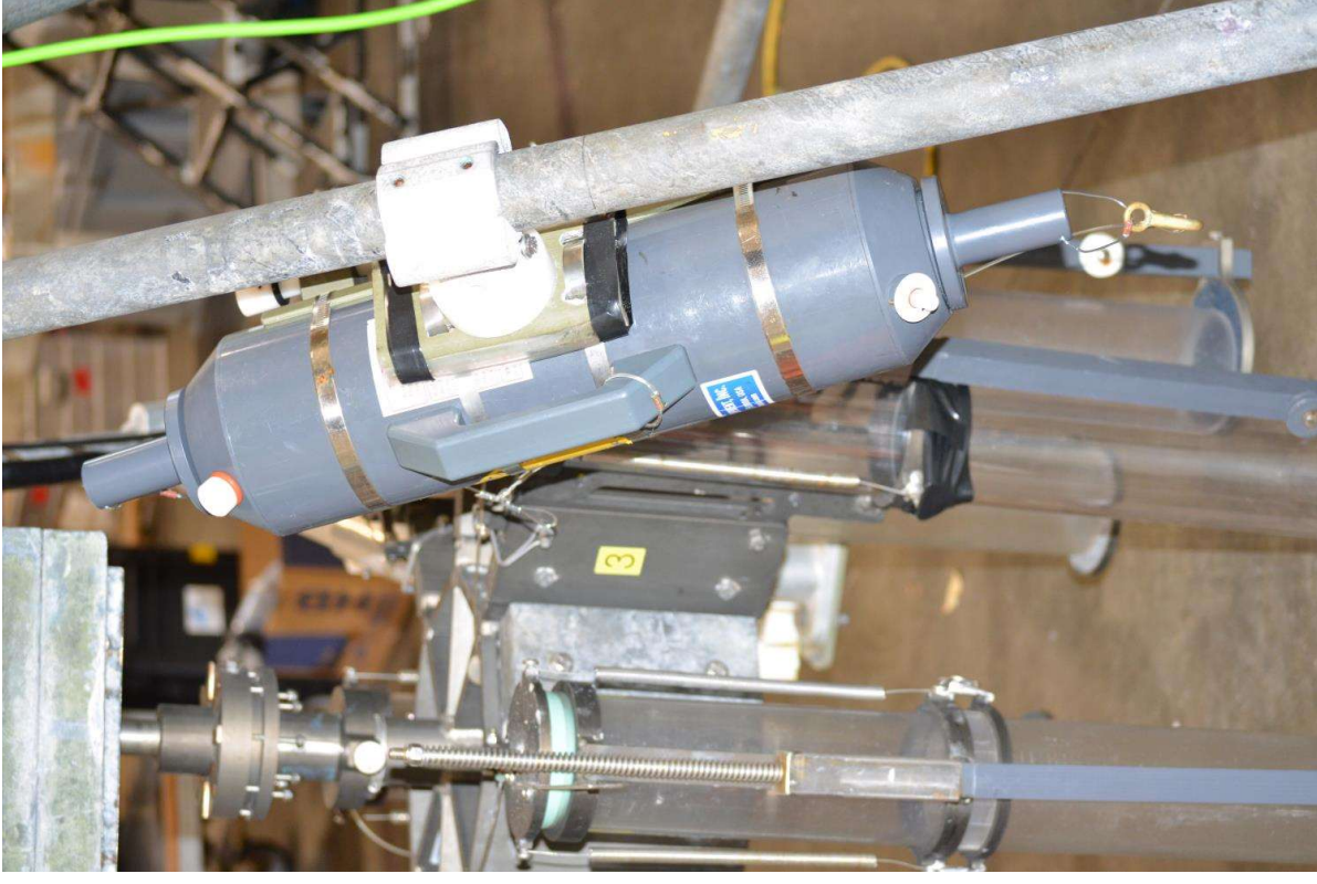
(left) DSPL IP- multiseacam – HD video camera that monitors anti-pretrip collar and motor.
