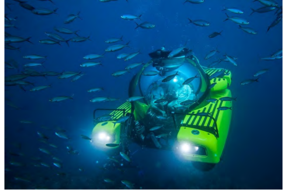
Figure 12: The HOVs Triton and Deep Rover are adapted from commercial vehicles, and are now capable of conducting a full suite of scientific measurements and samples.
