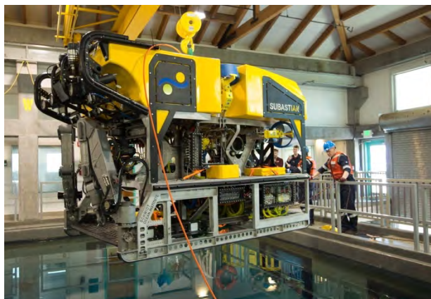
Figure 9: The ROV SUBastian is owned and operated by the Schmidt Ocean Institute, and is one of the newest research ROVs in the U.S., employing many of the latest imaging, propulsion, and sampling technologies. © Schmidt Ocean Institute
