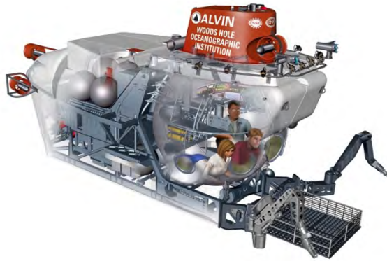
Figure 11: The HOV Alvin is the world's most accomplished submersible. The recent upgrade allows users to record HD video, run a suite of instruments, and –in the coming months- dive to 6500 meters. © WHOI
