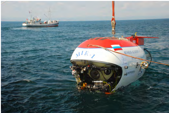
Figure 13: The HOVs Mir-1 and Mir-2 are deployed from the same surface vessel, allowing investigators the opportunity to have two vehicles on site. The Mirs have been used extensively in research, exploration, and film-making. © Russian Academy of Sciences.
