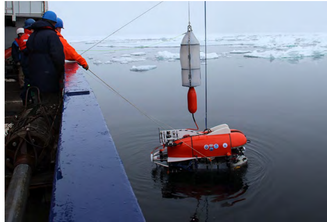
Figure 10: The hybrid ROV Nereid is specially designed for use under ice, enabling investigators to conduct experiments in regions inaccessible to traditional ROVs and HOVs. © WHOI.
