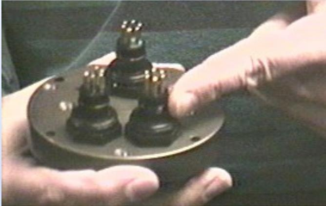
Lubricate molded ridge on bulkhead connectors with 100% silicone grease
