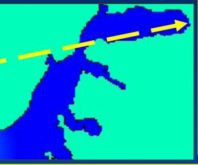
1. Tsunami signal arriving time without tide: 20 minutes and 50 minutes at high tide because of total depth increase and, respectively, increase of tsunami wave propagation speed.
