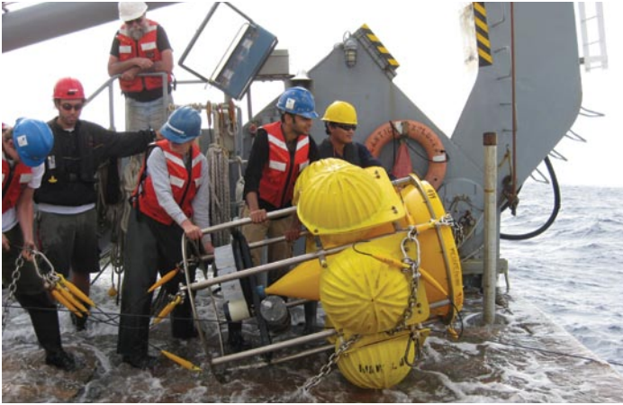
Researchers prepare for the deployment of the Oceanic Flux Program (OFP) time-series sediment trap mooring off Bermuda on the R/V Atlantic Explorer (BIOS).
