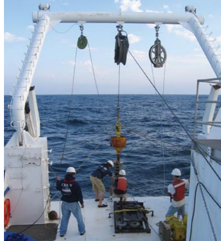
Preparing to deploy a sediment corer off the R/V Pelican (LUMCON).
