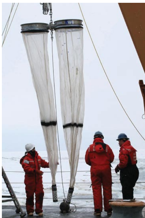
Bongo nets being deployed off of the USCGC Healy.
