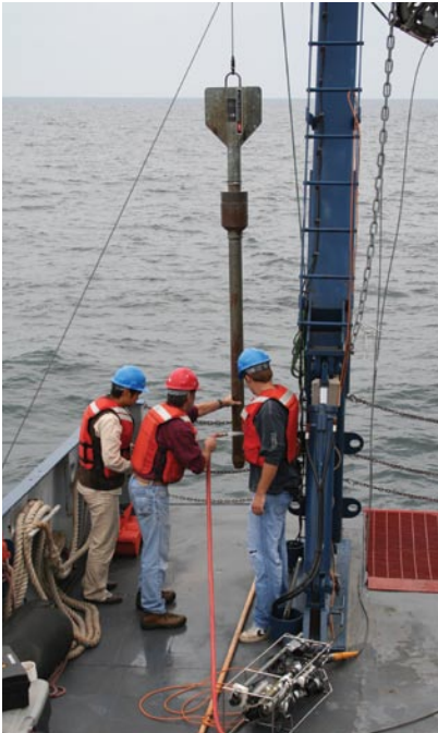
Gravity coring off the back deck of the R/V Blue Heron (U. Minn.).
