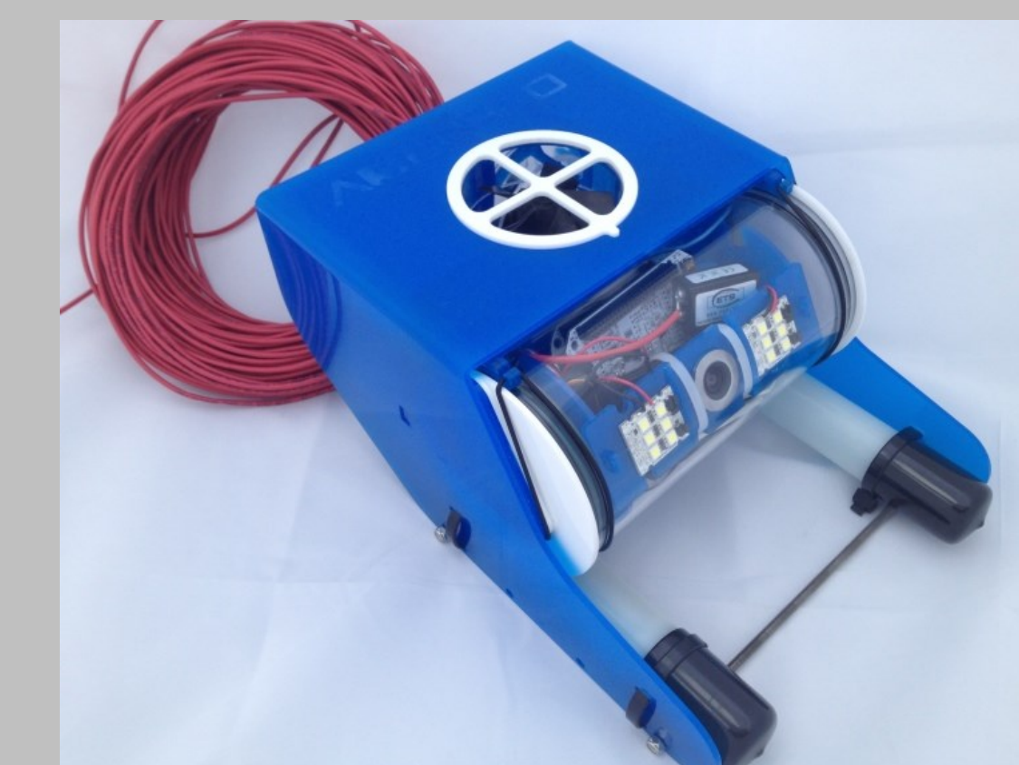
Figure 6. BeagleBone computer is used in this OpenROV project. [www.openrov.com]
