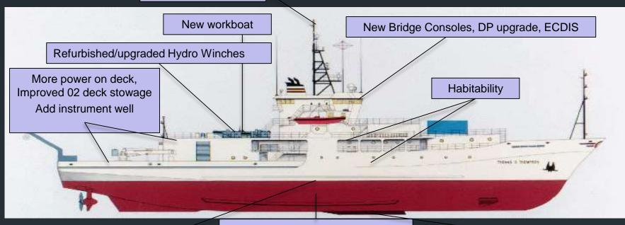
Lab Lighting / Decks / Ventilation Remove Hydro-Sweep, new Electronics Space with dedicated cooling **RE-POWER** – new engines, alternators, propulsion motors, switchgear, drives, AMS, controls
