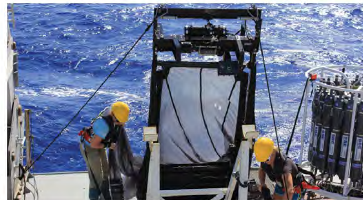
Students were trained on the Multiple Opening/Closing Net and Environmental Sensing System (MOCNESS) to collect zooplankton samples off Oahu on the third student cruise.
