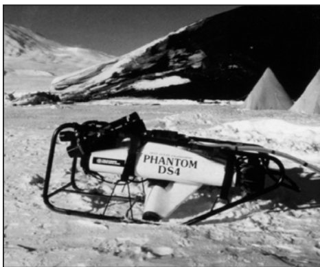
Photo 2: Deep Ocean Engineering Phantom is an example of a small electric ROV.
