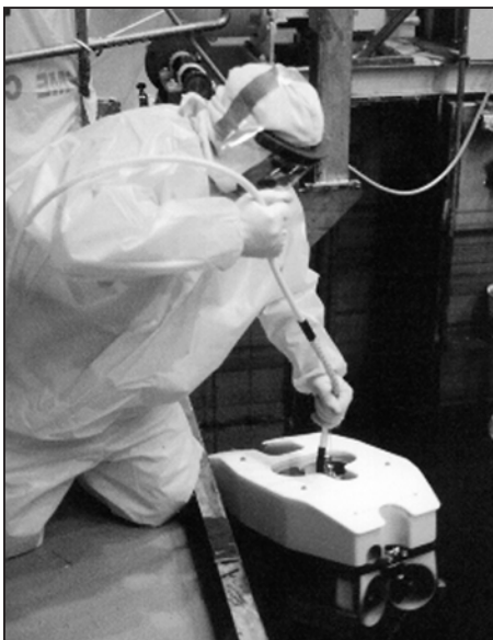
Pressurized Water Reactor ROV, the PI50, is launched to conduct a nuclear power plant inspection.
