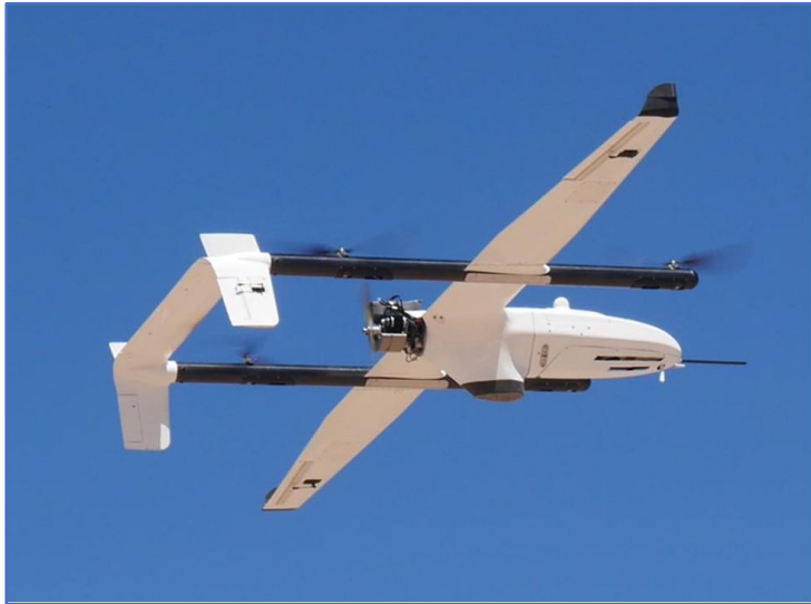
L3Harris FVR-55 with Clear Sky Payload onboard
