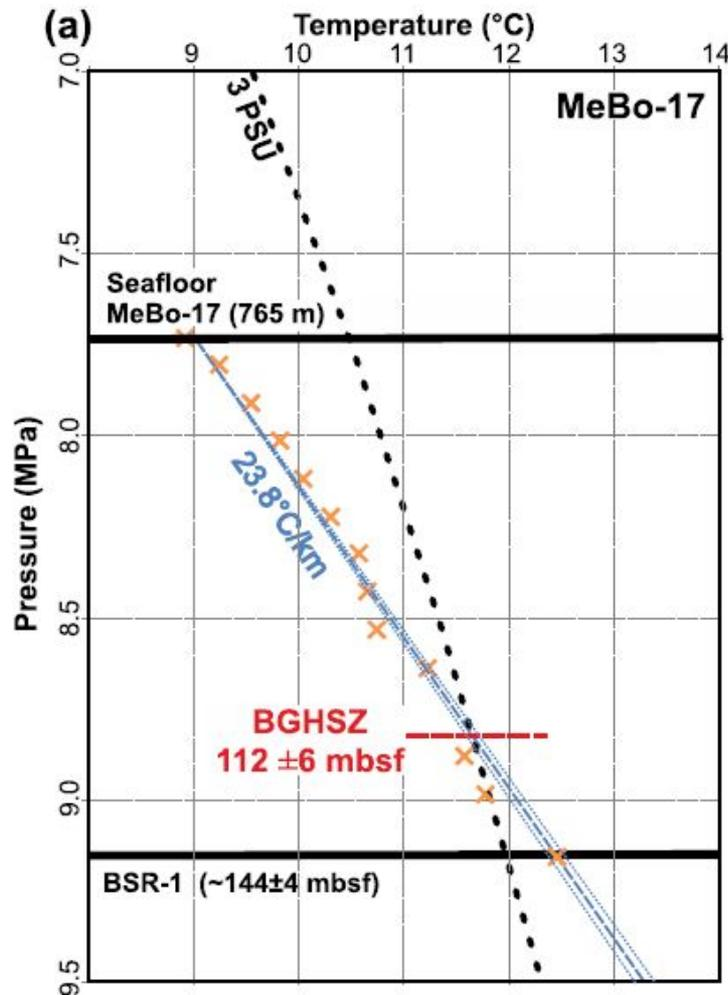
In-situ borehole temperature measurements confirm dynamics of the gas hydrate stability zone at the upper Danube deep sea fan, Black Sea
