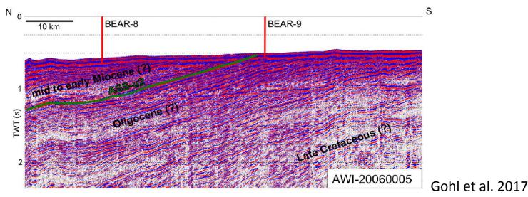
**Figure 5.** Seismic record from the middle shelf of the western ASE shows dipping older shelf sequence with a presumed stratigraphic age and unconformity ASSu2 from Gohl et al. (2013). The Parasound records on top show some of the dipping layer boundaries of the sequence overlain by a thin glacial and postglacial drape at drill sites BEAR-8 and BEAR-9. The vertical axes in both record types are two-way traveltime (TWT).
