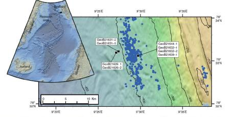
Fig. 1 Location of coring sites and gas flares. Gas flares (blue dots) were identified during a previous cruise<sup>11</sup>. Locations are listed in Supplementary Table 1
