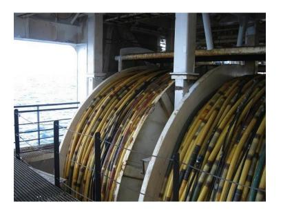
Langseth Maximum Array: 4 hydrophone streamers 6 kilometers long each
