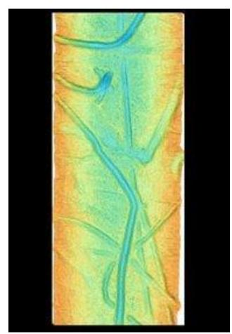
Processed multibeam data, showing iceberg gouges on the Chukchi Shelf. The depths are color-coded: Blue is deep and red is shallow.
