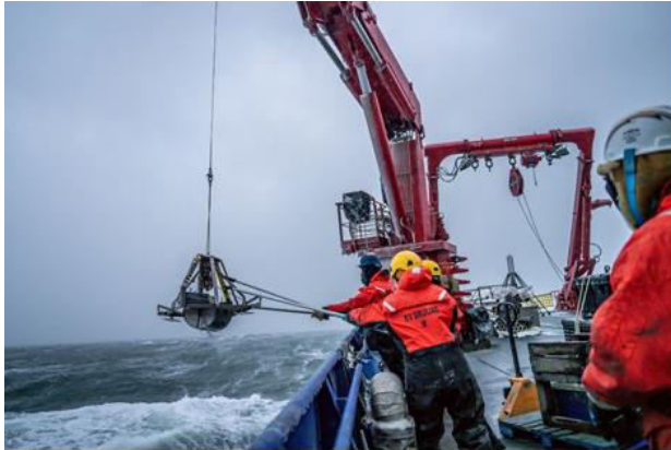
Battelle ARO supported Lloyd Pikok Jr onboard the R/V Skuliaq as the remote community contact for the cruise conducting outreach from the vessel. His daily updates shared images like this from the cruise. The science and deck teams perform in Van Veen Sediment Grab in Arctic Conditions. Photo: Amanda Kowlaski
