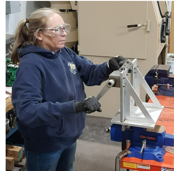
1/4", 3/8", 9/16" 3 x 19 Wire Rope Mandrel Wrap Test
