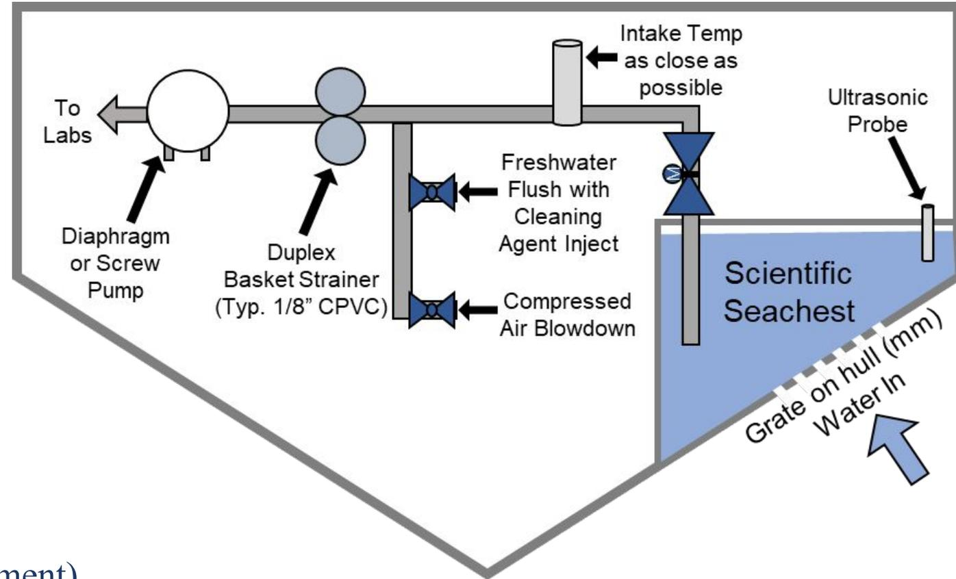
Flow-through system schematic, K. Watkins-Brandt
