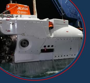
6500m depth rated DSV, capable of large payloads with an extensive sensor and imaging suite.
