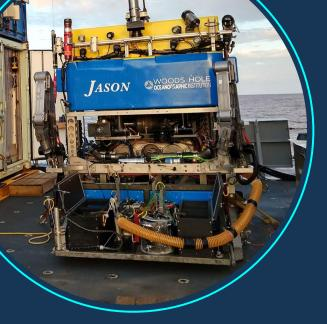
Jason is a remotely operated vehicle (ROV)
